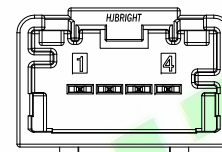
4 CIRCUIT RIGHT ANGLE HEADER POLARIZATION OPTION C TYPE COLOR:DARK GRA
